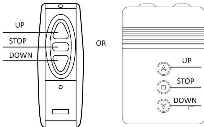
The electric projector screen can be controlled by the included dual remote system (IR or RF). Both remotes can be used to control the screen.
